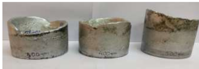
Fig 3.3. Cast of 8mm thickness of Al 5% Si with 1% Zirconia reinforcement
