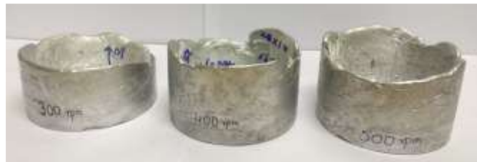
Fig 3.1. Cast of 4mm thickness of Al 5% Si with 1% Zirconia reinforcement
